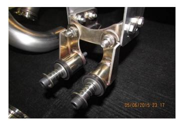
The image below is the installed mount after the system has been warmed up (notice the springs are slightly compressed) Expect the springs to be completely collapsed when the system is at operating temperature.
