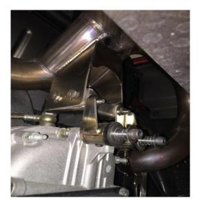
This image represents the SCUD model. Notice the aluminum drop brackets are vertical. Thus the aluminum drop brackets must be lock tight(ed) and tightened prior to installing the bushing portion of the mount(s) Please refer to instruction 5 again as a reminder
